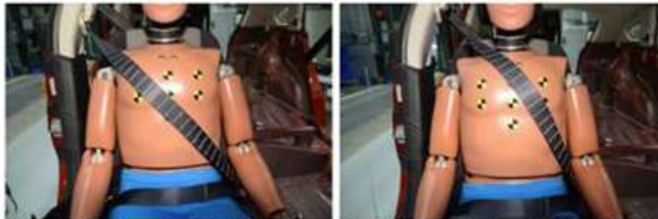
Figure 7. Belt Routing 50th Male Dummy D-ring Down (Left) and D-ring Up (Right)
