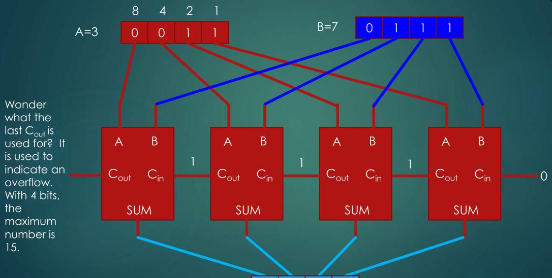
While this design works, we need to wait for the carry to propagate through the circuit. A Carry Look Ahead circuit is used to resolved this problem.
