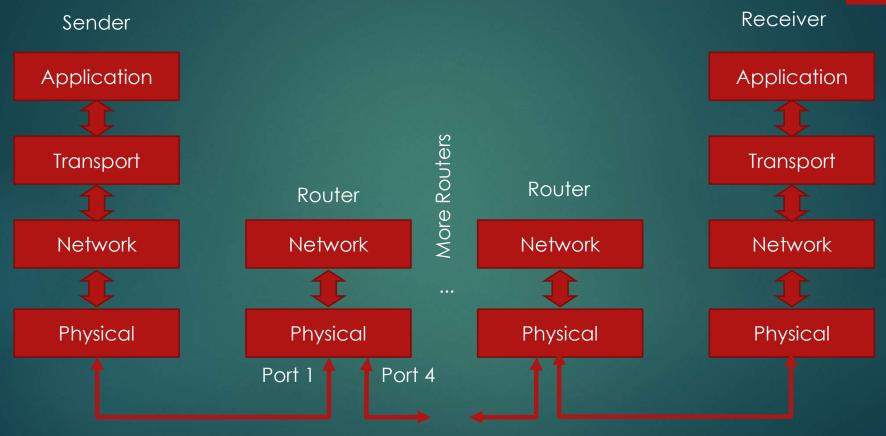
Routing table will determine which port will be used on the router
