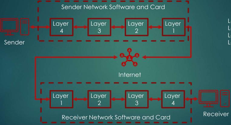
Layer 4 Application Layer 3 Transport Layer 2 Network Layer 1 Physical
