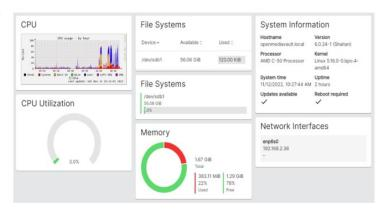
For example, we can see at a glance that the NAS at idle is using very little (3%) of the available CPU processing power, and only a moderate amount (22%) of the system memory. Only a single text file (120 KB) has been stored on the 64 GB flash drive so the storage disk utilization is less than 1%.
