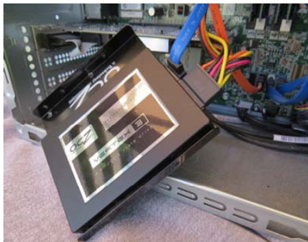
Figure 1. SSD for a desktop computer
