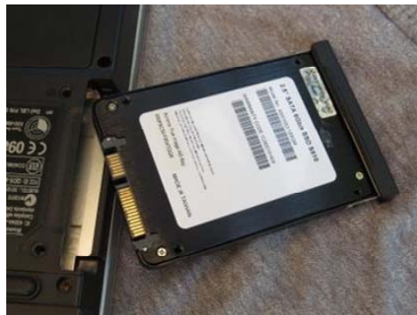
Figure 2. Inserting an SSD into a laptop’s drive bay
